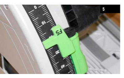
Set the plunge saw to the cutting depth that corresponds to the thickness of the board to be cut. In the case of a board with a thickness of 14 mm (9/16"), set the device to a cutting depth of 15 mm (19/32").
