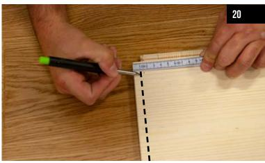
Mark a line on the bottom layer, from the end part of the removed 5Gc lock, along the entire width of the board at a distance of 16 mm (5/8") from the front edge.
